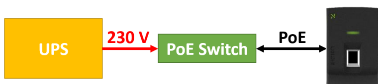
Obr. 5: PoE switch s UPS
